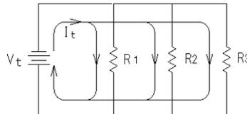
Fig.2 Example of a parallel circuit.
